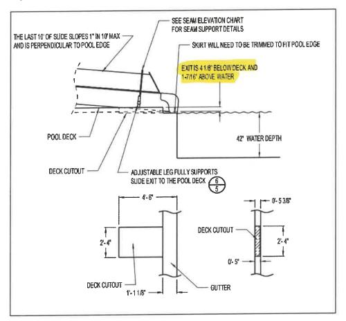
5. 15.5(17) Water slide flume locations are not dimensioned. Provide dimensions confirming spacing is provided in accordance with 15.5(17)a(4).
